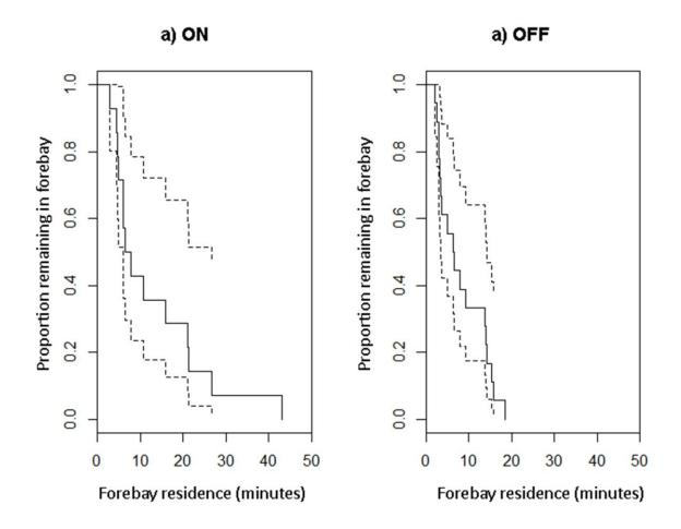
Figure 3 Estimated Kaplan-Meier curves and 0.95 confidence intervals (dashed lines) describing forebay residence times (minutes) of downstream migrating eel passing the intake (n = 32) under the (a) ON and (b) OFF infrasound treatments
