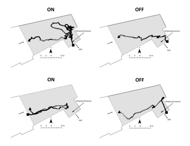
Figure 4 Example trajectories of four downstream-migrating adult eel through the forebay of a former hydropower facility when an infrasound source (11.9 Hz) was turned ON and OFF. Black triangles and squares denote the start and end of tracks, respectively.
