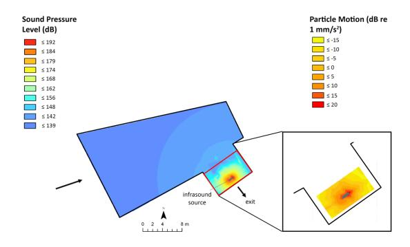
Figure 2 Sound pressure level (dB) and particle motion (dB re 1 mm/s²) (inset) in the forebay of a redundant hydropower facility under the ON treatment when the infrasound source was emitting at 11.9 Hz. The red outline denotes the perimeter of the intake channel. The arrows denote principal flow direction.
