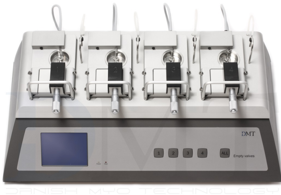
Figure 2.1: The wire myograph system. A Danish Myo Technology (DMT) multi-wire myograph was used to generate contractile data from vessels and segments throughout this project. Image taken with permission from DMT.
