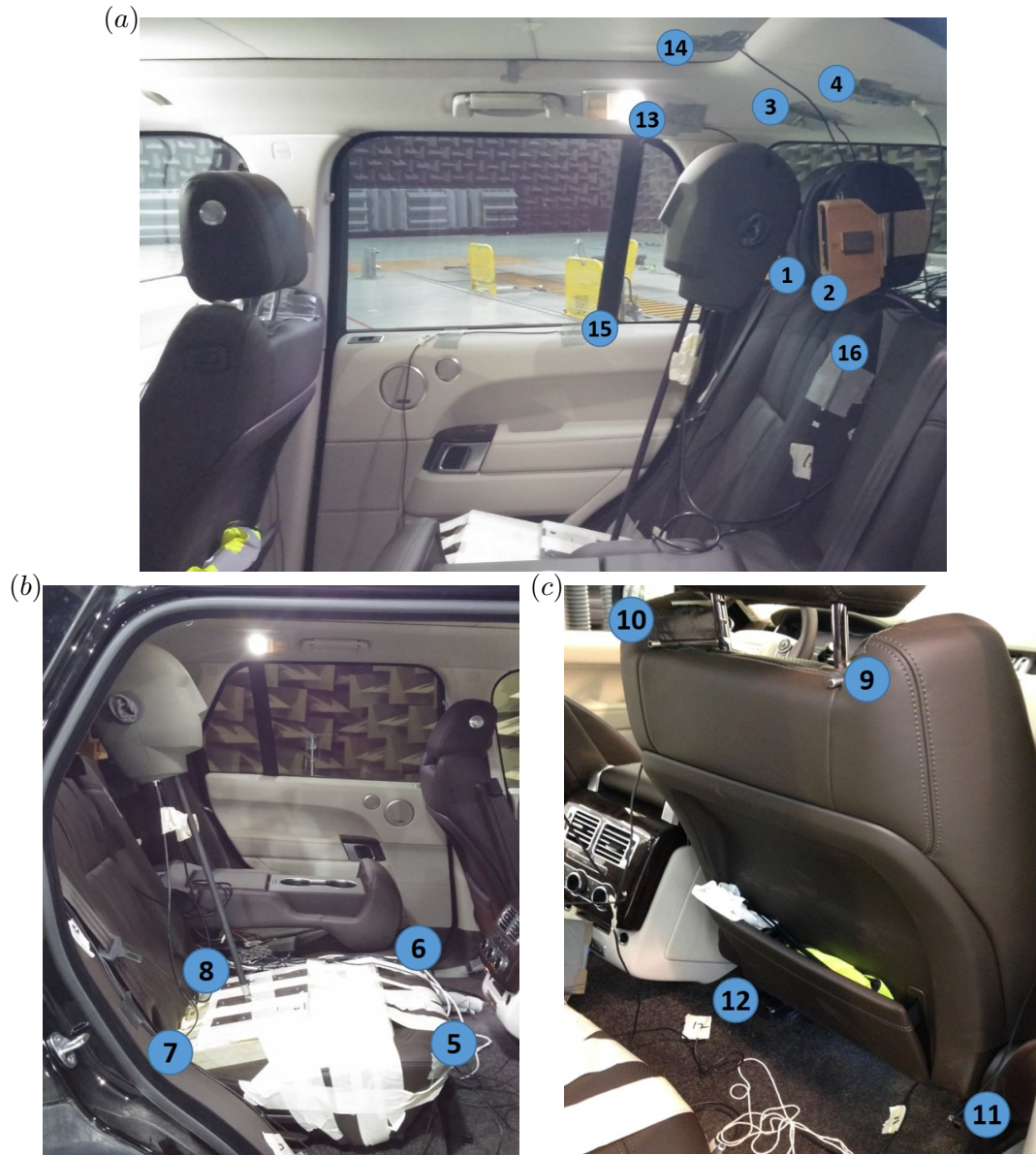
Figure 8.1: The overall installation for the remote microphone technique and local active sound control experiments when interior road noise is measured at the rear right seat of a large SUV using 16 potential positions for monitoring microphones around the dummy head and two error microphones in the ears of a dummy head. Eight potential monitoring microphones are positioned on the headrest and ceiling (a), four monitoring microphones on the rear right seat (b) and four monitoring microphones on the front right seat (c).
