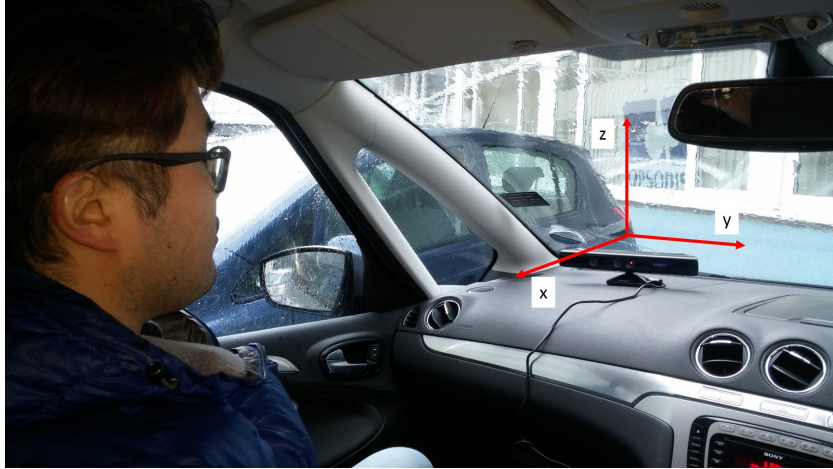
Figure F.1: The installation of a head tracking device, the Kinect on the dashboard inside a vehicle cabin for measuring head movements of an occupant.
