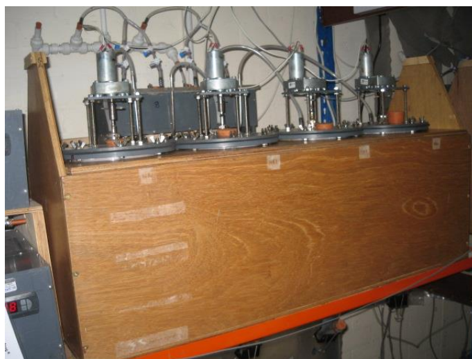
Set of 5 L digesters in temperature controlled box
