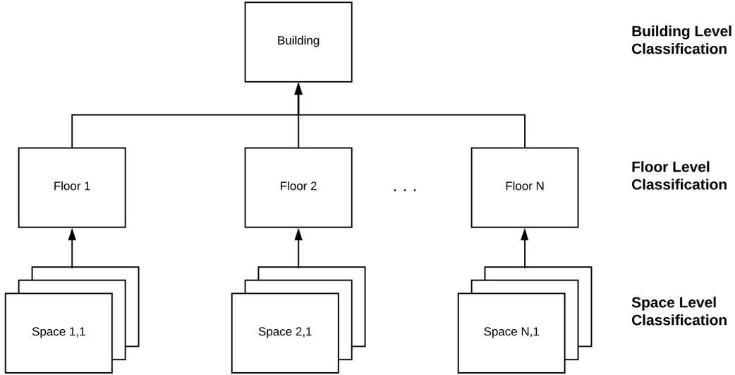
Figure 2: Bottom-up Design of the Building Rating System. The building accessibility assessment is started with the bottommost *Space Classification*, then *Floor Classification* using scores from the spaces' classification, and finally *Building Classification* using scores from the floors' classification
