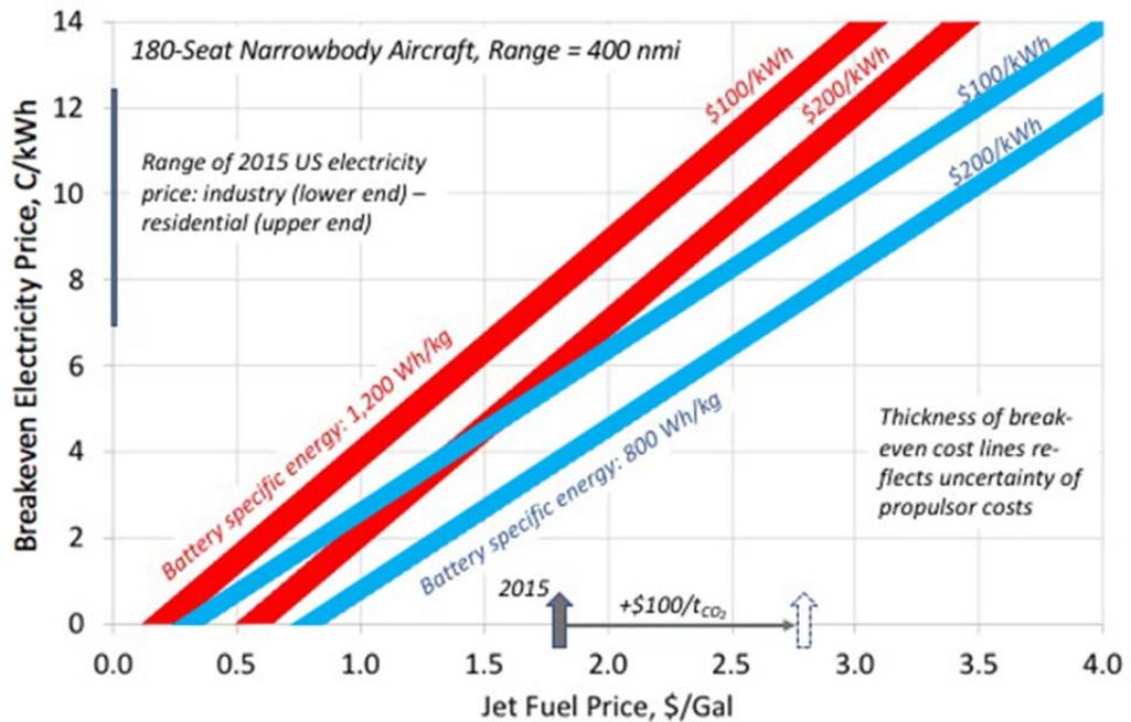
512 **Fig. 2.** Break-even electricity price for a first-generation all-electric aircraft. The reference jet
