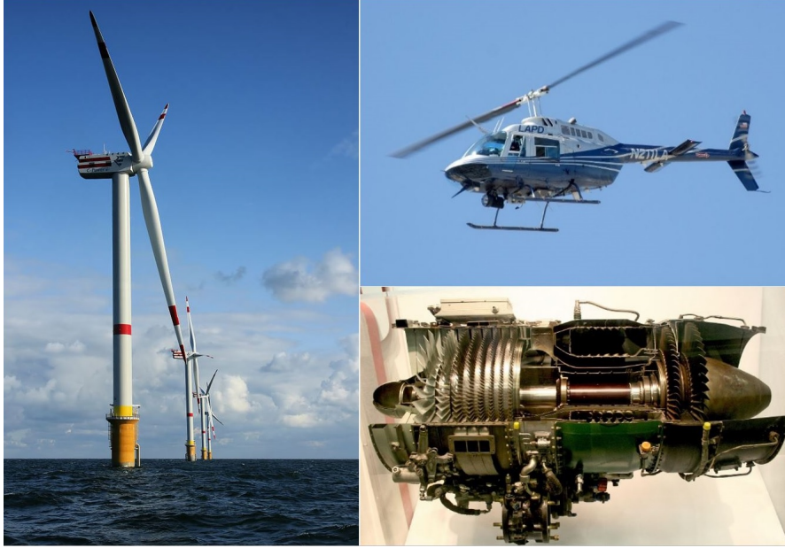
Figure 1.1: Applications of rotating beams. Wind turbine REpower 5M in the North Sea off the coast of Belgium Hillewaert (2008) . A General Electric J85-GE-17A turbojet engine (1970) Acharya (2008) . Bell 206 Jetranger helicopter Field (2006) .
