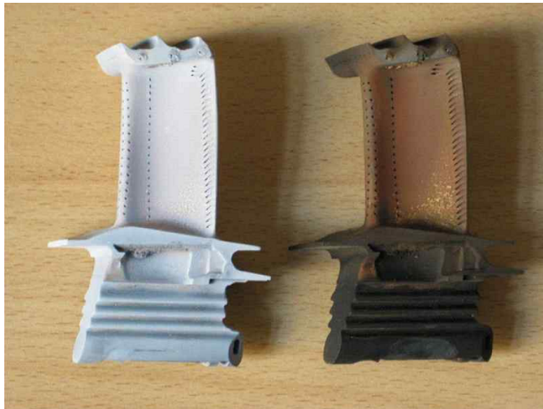
Figure B.1: Example of a titanium dioxide coated, used turbine blade. This image is reproduced from the report by Heinze (2013).
