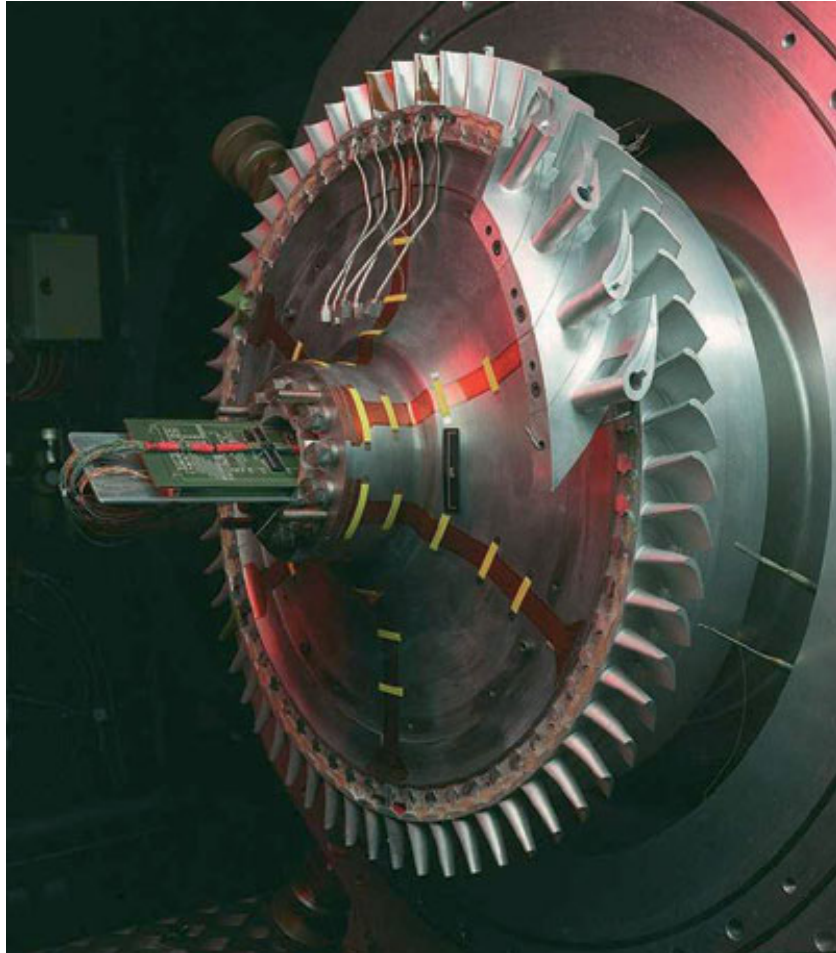
Figure D.1: MT1 turbine stage test bench at QinetiQ (source: see footnote 1 )
