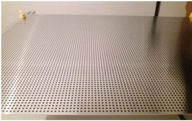
Fig. 1 Printed grid, pitch of 7.14 mm
