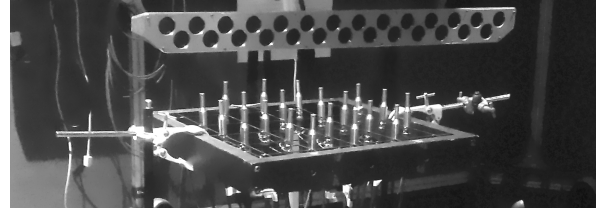
Fig. 1. Foreground: 20-channel microphone array; Background: 27-channel loudspeaker array.
