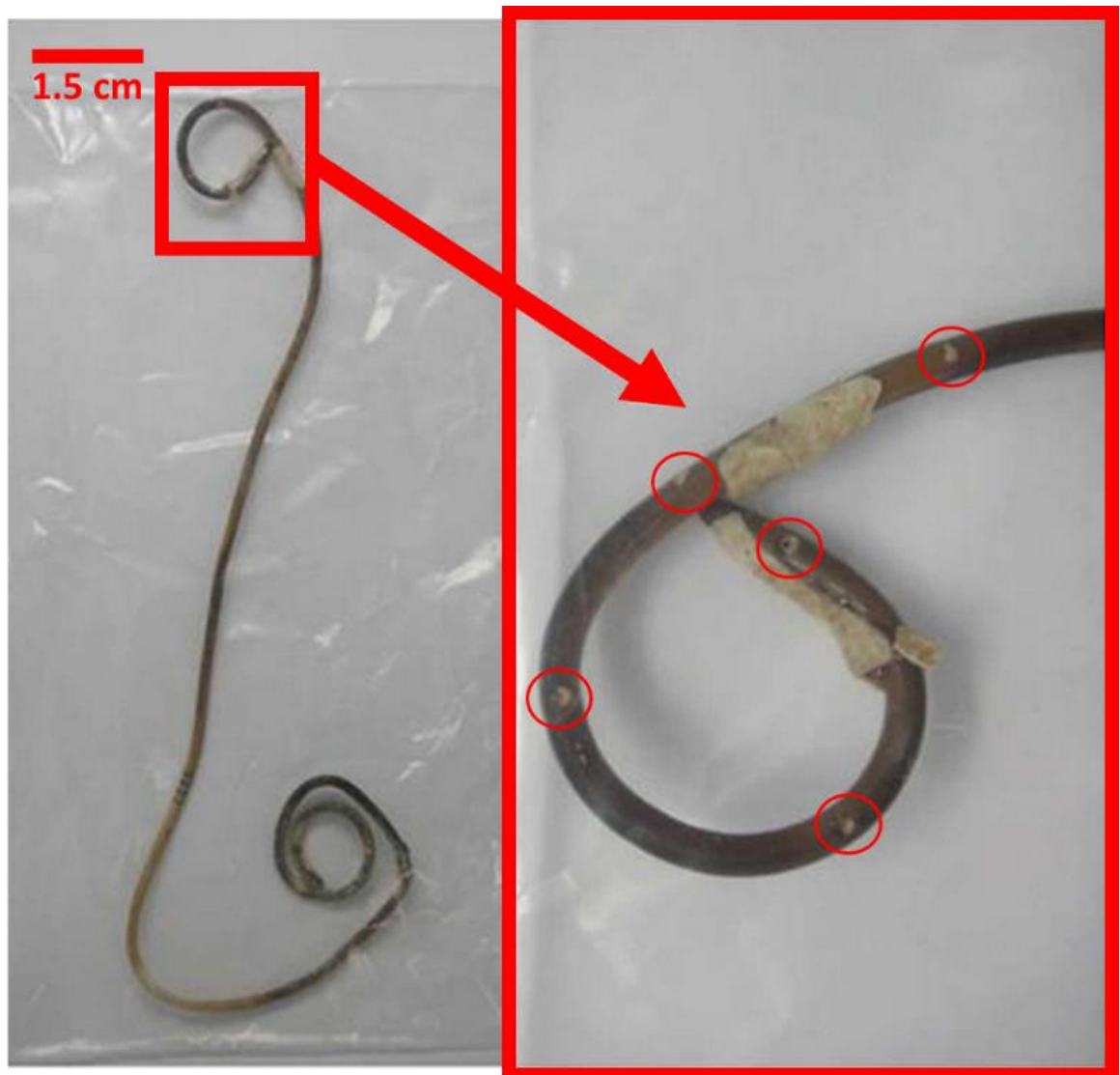
Figure 1-5 Photograph illustrating samples of encrusted ureteral stents retrieved after 6 years from an 88-year old patient. The red circles indicate complete blockage of side-holes after long-term stent deployment. The image has been taken from Gu et al. [55], with minor adaptations. Stents have approximate dimensions of 1.5 mm × 2.5 mm (ID × OD).
