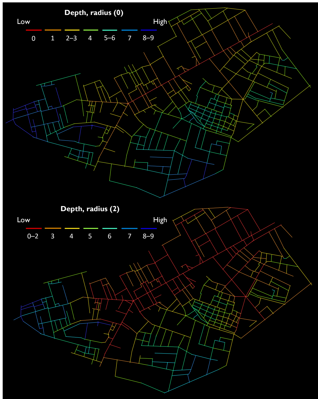
Figure 5.4 Axial graphs showing different step depths (e.g. turns) from the decumanus (Top: step depth – 0; Bottom: step depth – 2).
