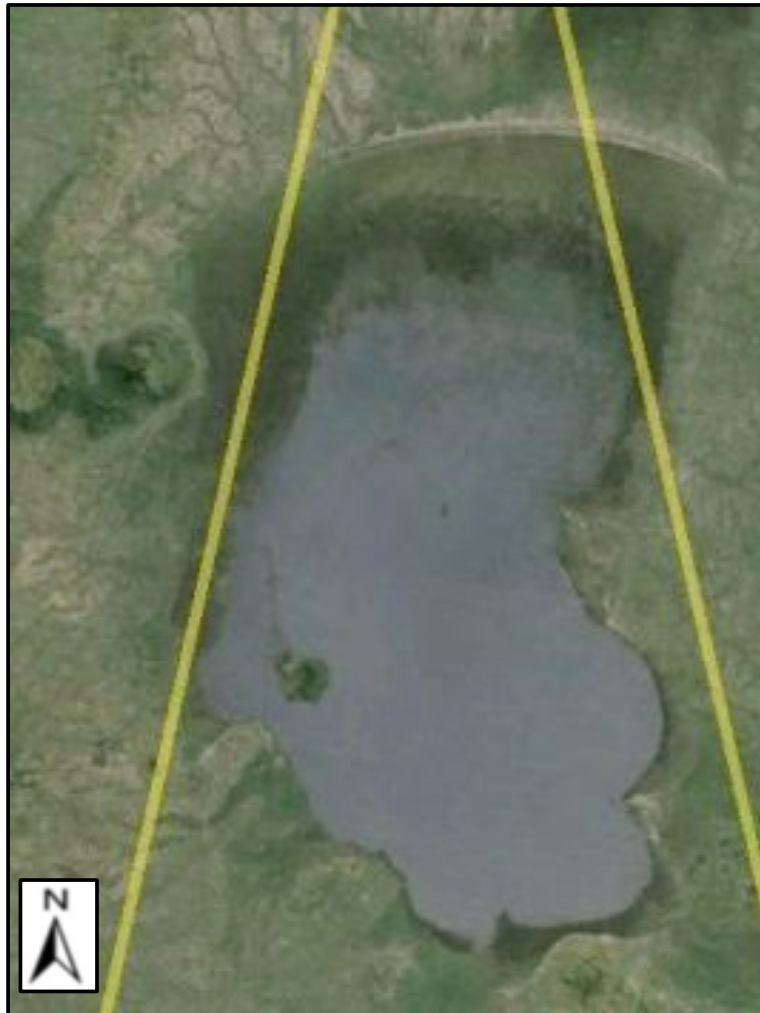
Figure 4-1 Google Earth optical imagery of the ENVISAT ascending (rev571/pass285) and descending (rev184/pass092) pass over Lake Chilwa, depicted in yellow.
