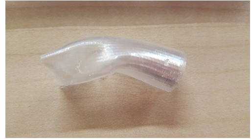
PC tube after annealing for 30 minutes at 200 °C .
