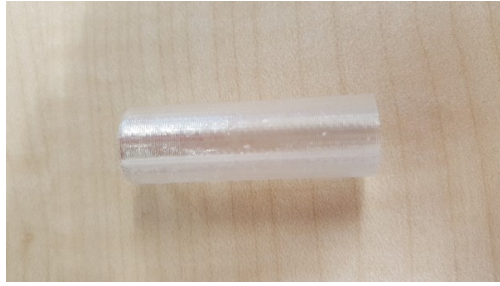
PC tube after annealing for 30 minutes at 125 °C .
