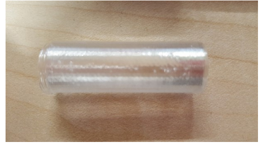
PC tube after annealing for 30 minutes at 150 °C .
