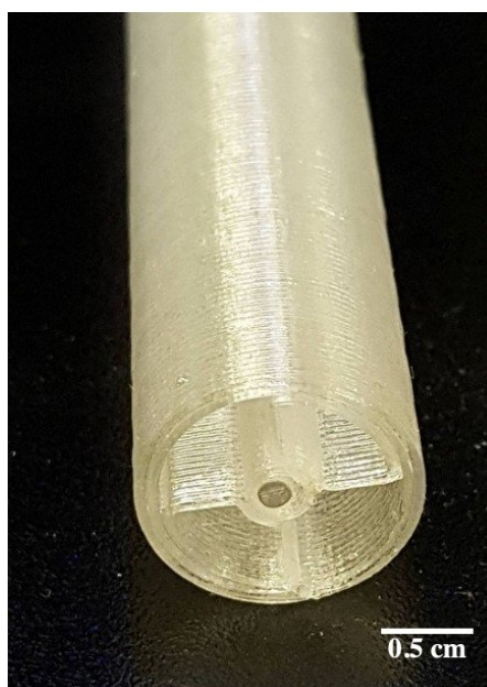
FIGURE 4.14: Cross-section of drawn PC wagon wheel preform printed using surface setting with filament inserted into the core to create a solid core.
