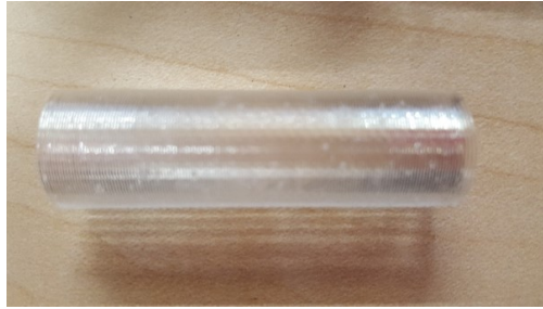
PC tube after annealing for 30 minutes at 175 °C .
