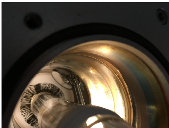
FIGURE 4.3: Susceptor installed in the drawing tower to enable the use of lower temperatures during the drawing process.
