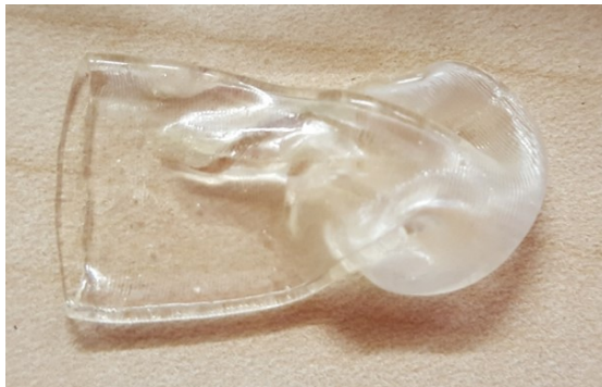
FIGURE 4.21: PC tube after annealing for 72 hours at 175 °C .
