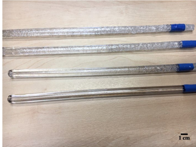
FIGURE 4.18: Four different Polycarbonate tubes all extruded from the same rod under the same conditions.
