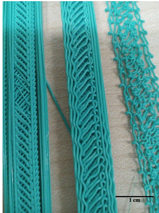
FIGURE 4.1: Three printed samples with different printing bed alignment settings. The distance between the nozzle and printing board was 0.5 mm, 2.5 mm, 5 mm from left to right.
