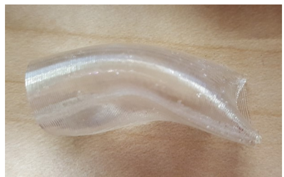
FIGURE 4.22: PC tube after annealing for 6 hours at 175 °C .
