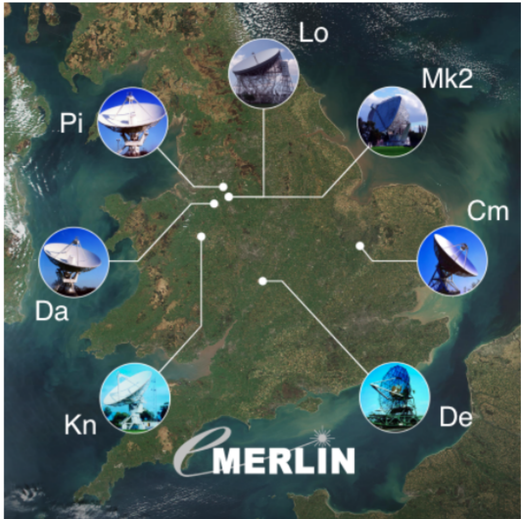
Figure 1.9: A geographical representation of the e-MERLIN array, showing that the antennas are spread across the UK and that e-MERLIN is an asymmetric array. This image is from the e-MERLIN website, www.e-merlin.ac.uk . For scale, the longest baseline is 217 km long which is between the Lovell and Cambridge antennas.
