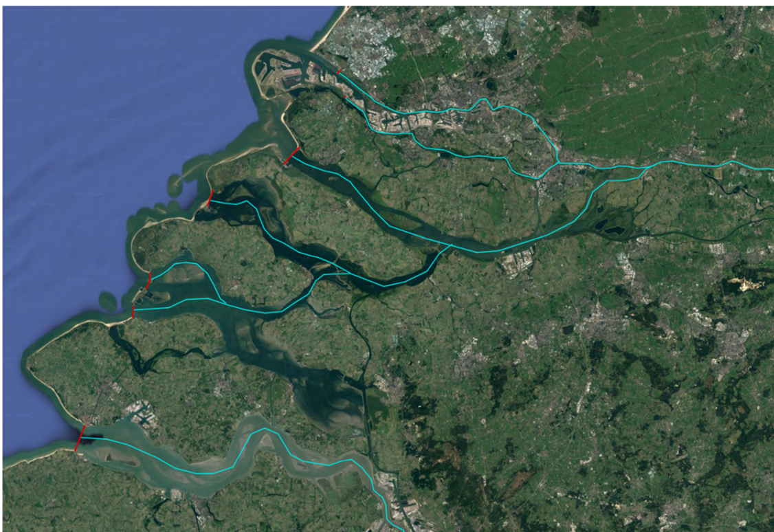
Figure 4: Proposed river distributaries and surge barrier positions as illustrated for the southern Netherlands.
