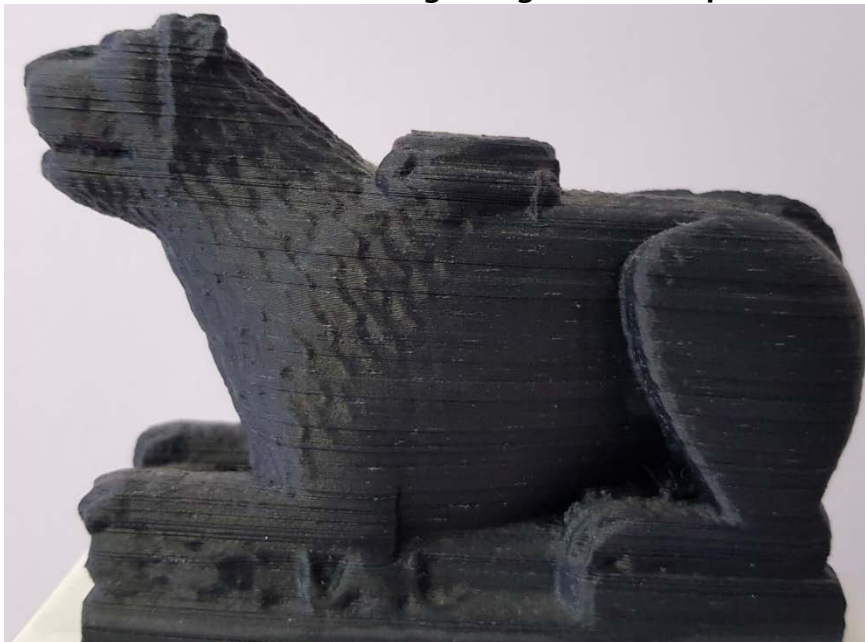
Figure 3 - 3DM of the Lion Column Base. The 3DM is printed of Black PLA plastic and is scaled and is 10×3×8cm. The original is exhibited in Parma Museum.
