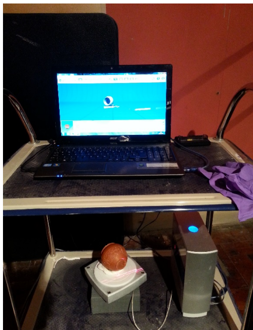
Figure 44 - Scanning using the 'Next Engine 3D'
