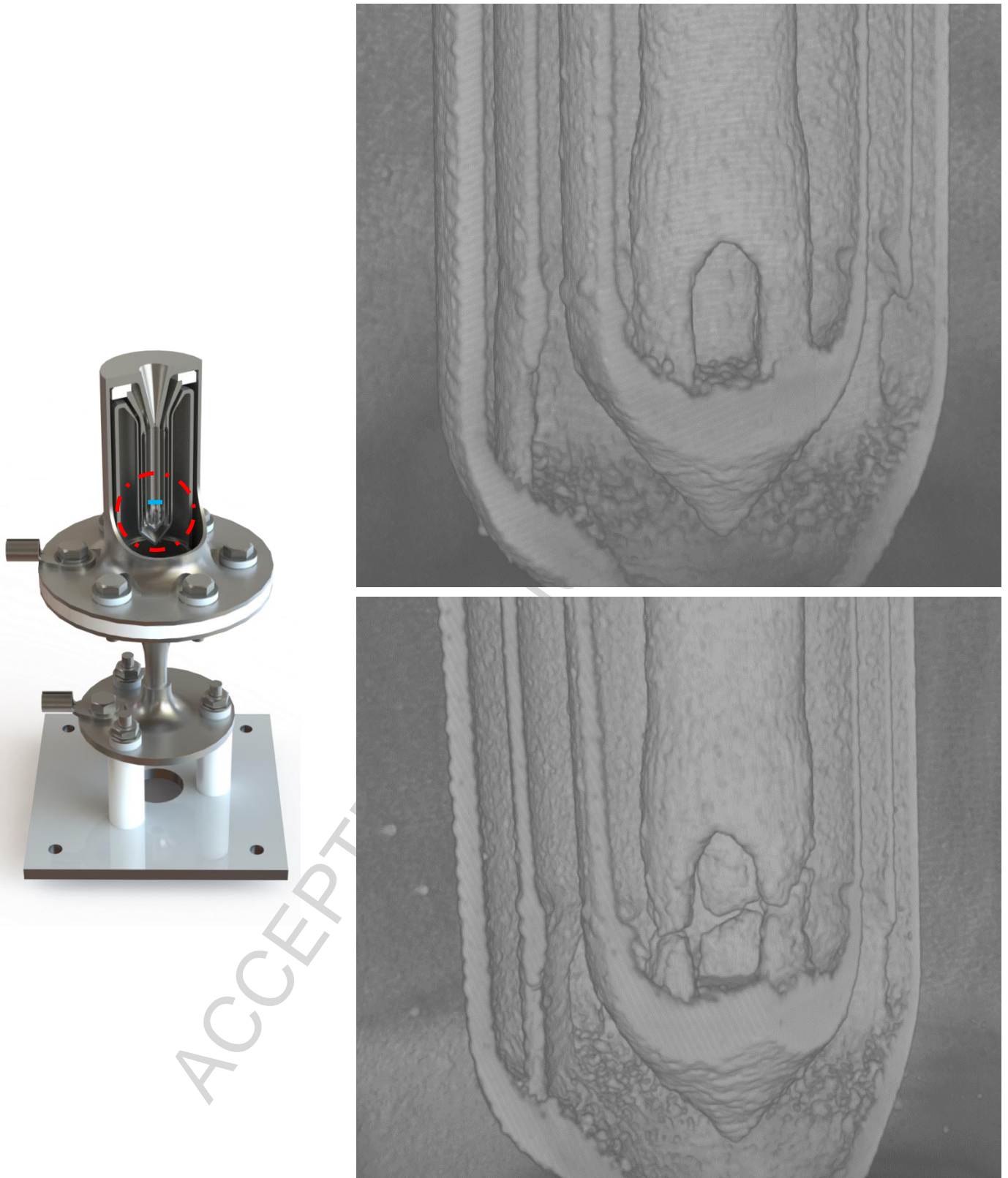
Figure 17: Left: Cutaway of thruster assembly. Red outline shows CT region of interest, and blue line shows location of optical micrograph in Figure 18. Right: Cutaway of 3D CT reconstructions of STAR-0-C before (top) and after (bottom) testing. Connecting struts at centre of image are intact before testing, and fully fractured after.
