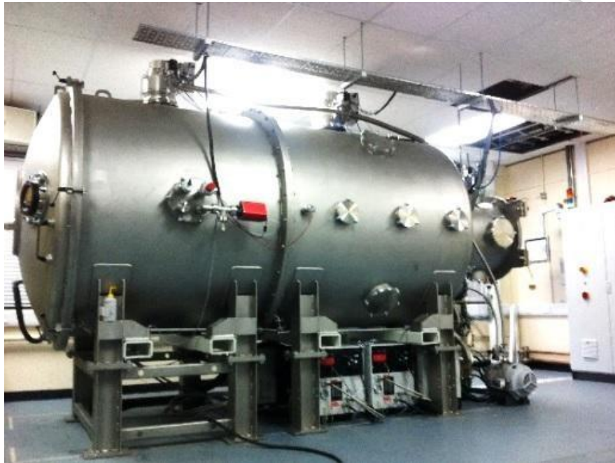
Figure 4: David Fearn EP Laboratory, vacuum chamber shown in centre.
