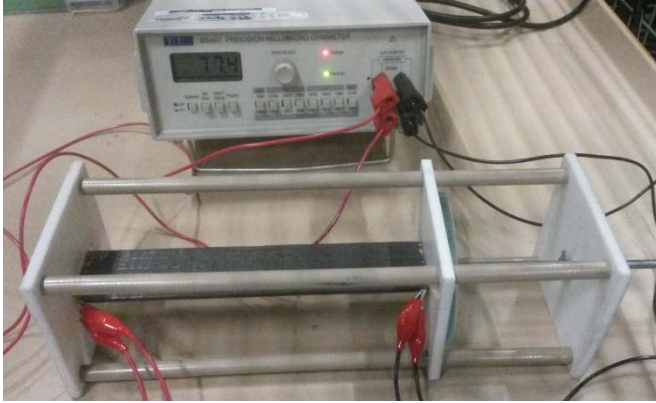
Figure 3: Experimental setup for transverse direction measurements.
