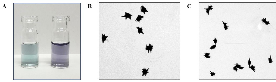
Figure 6.4. Characterisation of single and dimer branched gold nanoparticles A) Photography of the final products after growing single seeds (left) and dimer seeds (right) B) Transmission electron microscopy image of single grown branched gold nanoparticles and C) Transmission electron microscopy image of dimer grown branched gold nanoparticles. Scale bars are 100 nm
