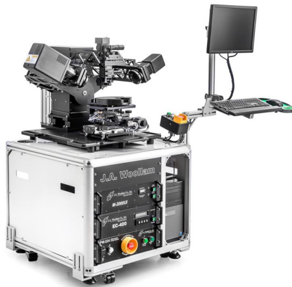
Figure 3.8: The ellipsometer (M-2000 TM , J. A. Woollam Co.) at SNC.
