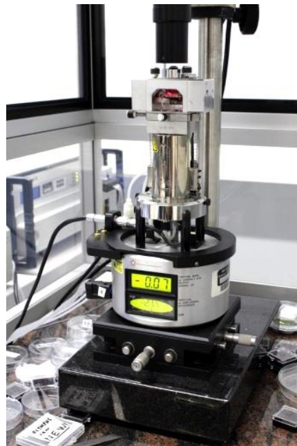
Figure 3.10: AFM (Multimode TM V, Veeco) in the Measurement Lab on a suspended workbench.
