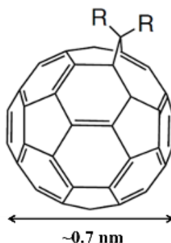
Figure 6.1: Molecular diagram of generic mono-adduct methanofullerene derivative resists. R represents the attached side chains to the C 60 molecule.
