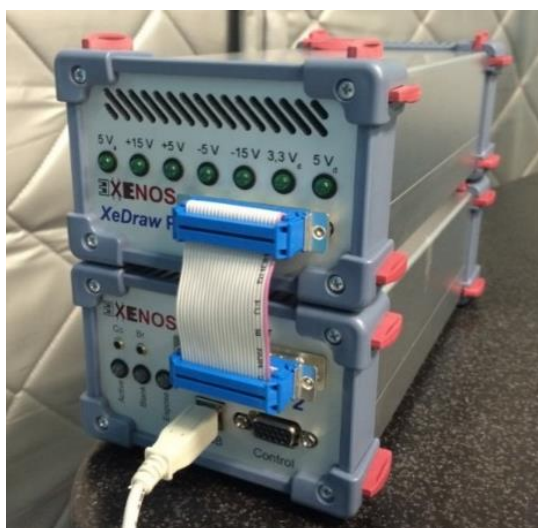
Figure 3.5: The external pattern generator of HIM system: XENOS Pattern Writer XeDraw2.
