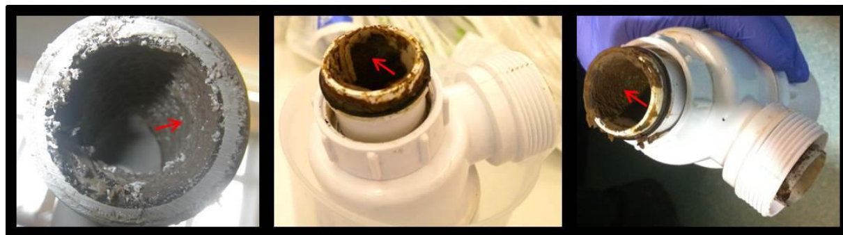
Figure 6.9 Visible biofilm in hospital sink waste traps. Red arrows indicate accumulation of biofilm. Traps (n=3) were sent to Public Health England, Porton Down. Photographs taken and provided by Ginny Moore (Public Health England).
