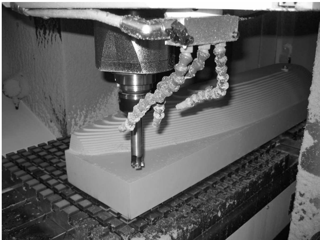
Figure 4 CNC machining of Victory model
