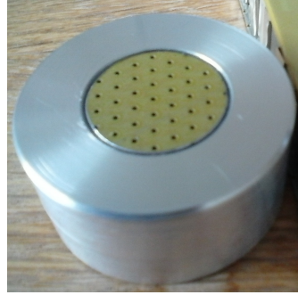
Figure 3.9: Punched aluminium SDOF sample extracted from the panel and inserted on the sample holder.
