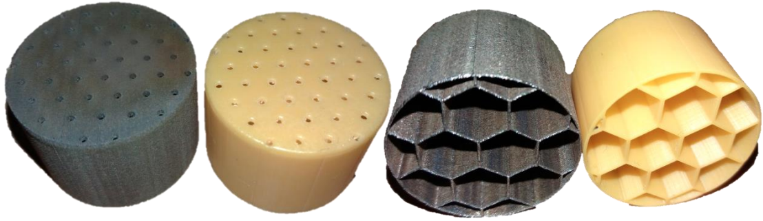
Figure 3.22: Laser sintered sample S1M on the left of each pair, and photopolymerized sample S1C on the right.
