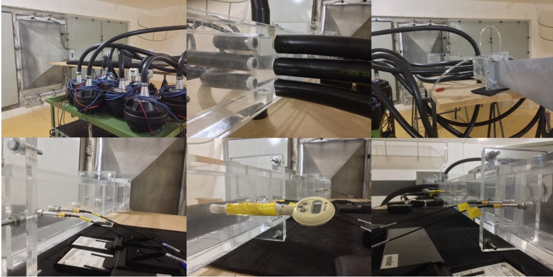
Figure 3.33: UFSC impedance test rig in operation. Nozzle and compression drivers on the top left, rubber tubes connected to the upstream section on the top center, diffuser and rubber tubes connected to the downstream section on the top right. Couplers with the microphones upstream, thermometer and microphones downstream are shown on the bottom left, center and right respectively.
