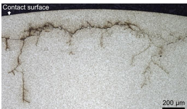
Figure C-6: Optical image of a typical WEC in the etched condition. Circumferential section, over-rolling direction right to left.
