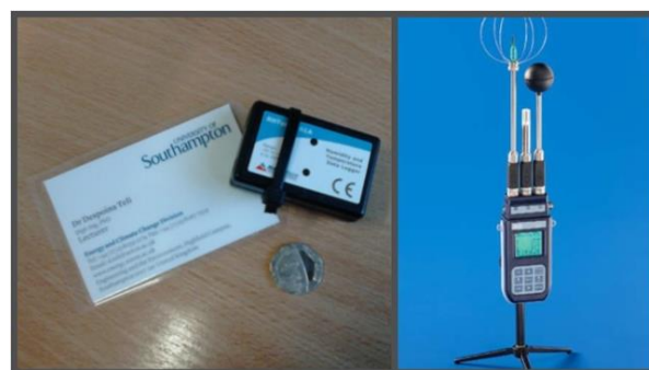
Figure 3.10 Image of MadgeTech RHTemp101A temperature and relative humidity data logger (left) and DeltaOhm HD32.3 environmental measurement kit (right) for air temperature, globe temperature, relative humidity and air velocity
