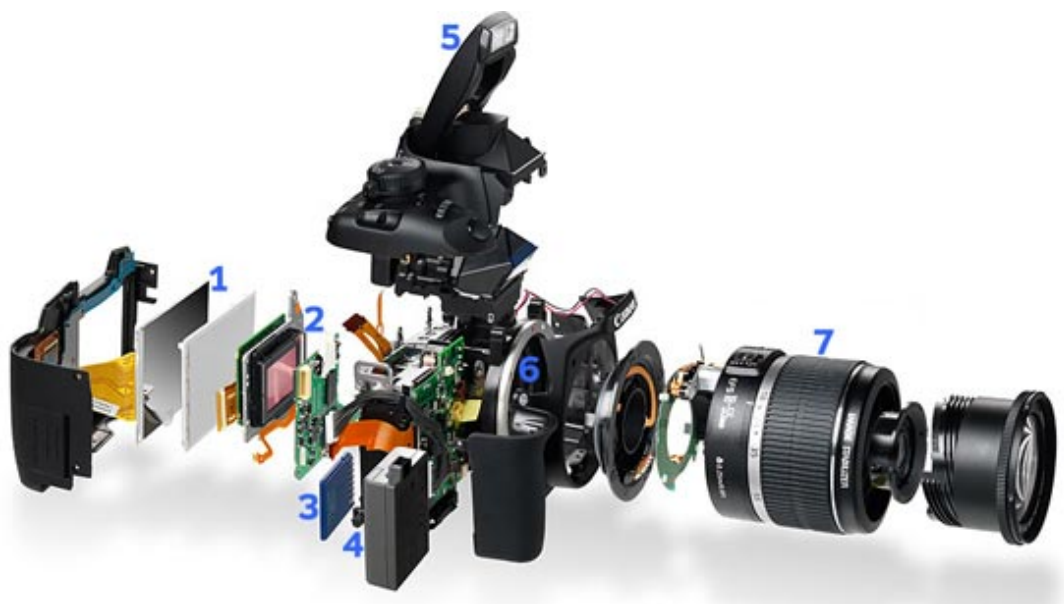
Fig. 11 Exploded view of a digital SLR camera
