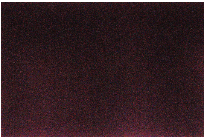
Fig. 24 Dark current image from a Canon EOS650 (22 minute exposure with lens cap on)
