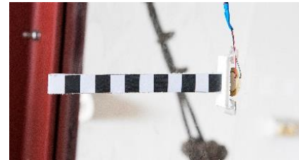
Figure 5. Deflection gauge used to track central deflection.
