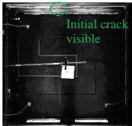
(b) Time of piezo transducer response ( t = t_c + 0.038 ms).
