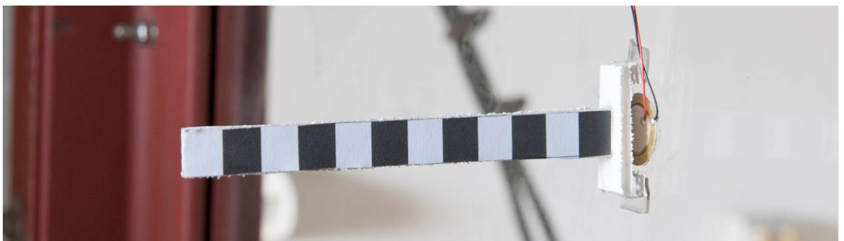
Figure 4.10: Deflection gauge tracked by cameras.
