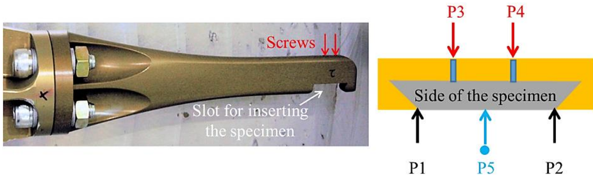
Fig. 8.16 Means of the specimen installed in the sample holder of WDE rig at NPL.
