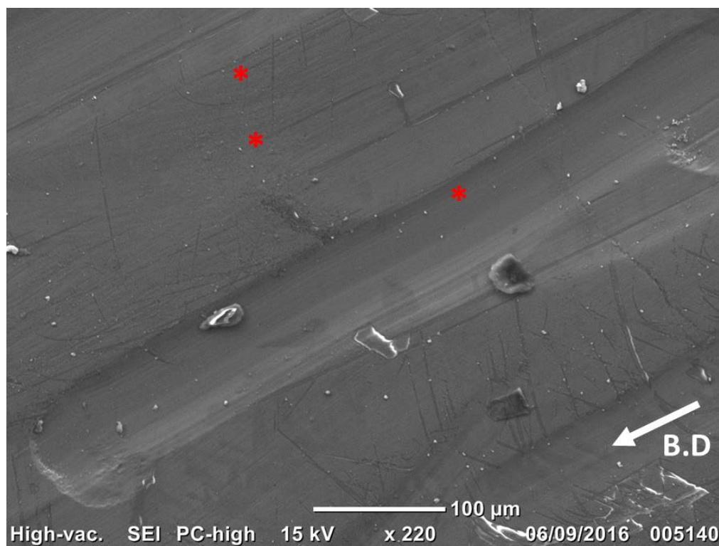
Figure 7.9: Bovine disc wear scar with GSK silica particles showing truncated groove indicated by the red asterisks.
