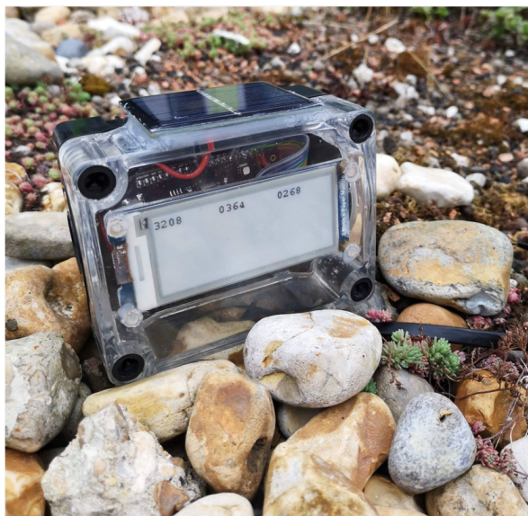
Figure 3. Photovoltaic technology provides a staple source of energy for a variety of energy-harvesting systems and is easy to implement as an addition to existing projects. This photo shows polycrystalline photovoltaic technology in use on an embedded sensing platform [36].
