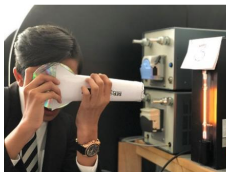
Figure X1 'Guess the Gas' workshop, illustrating concepts of spectroscopy through a built-it-yourself diffraction element [11].
