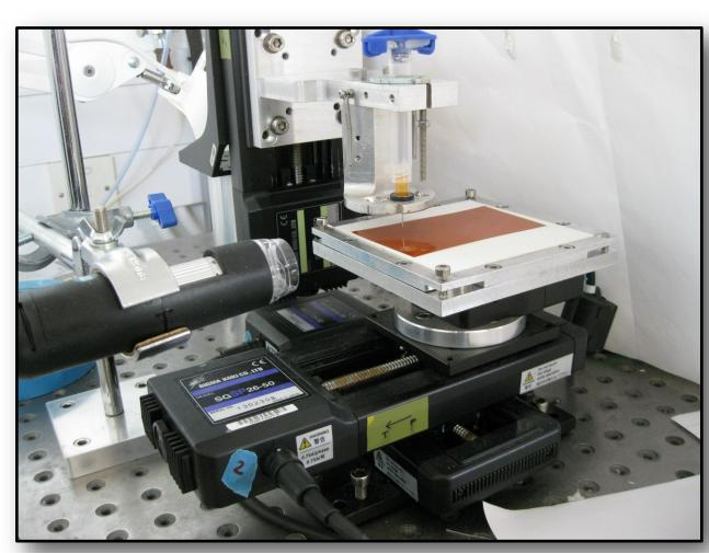
Pneumatic dispenser to control adhesive and encapsulation deposits
