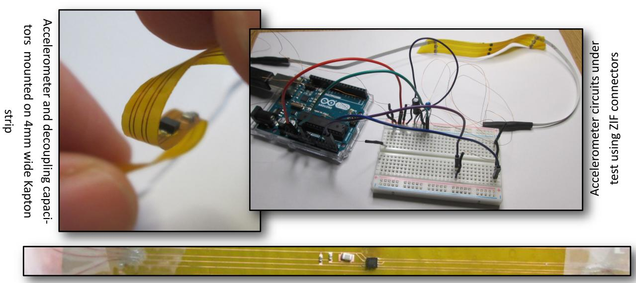
Accelerometer and decoupling capacitor circuit on 4mm wide Kapton strip
