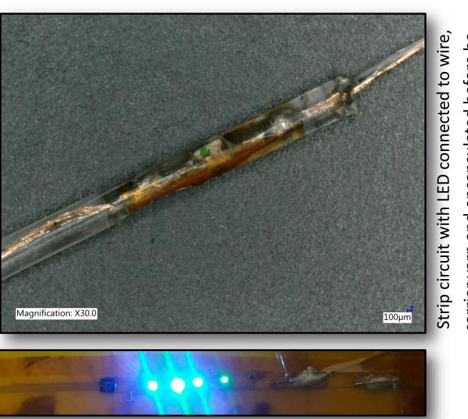
Temperature sensitive strip with LED output showing it is below the temperature threshold (blue output)
