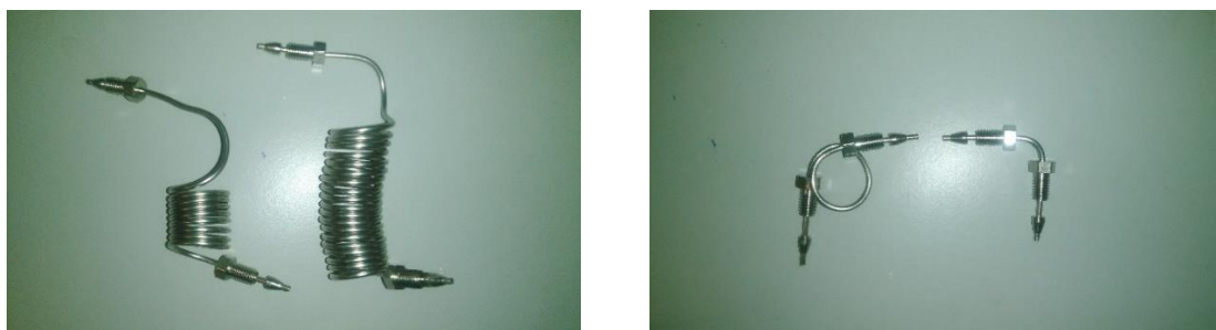
Figure 5.1: Micro-tube reactor ( \approx 100 \text{ cm} < L < 200 \text{ cm} ) used as pre-cooling loop (left), stainless steel micro-tube reactor ( L highly variable) used as reactor (right)
