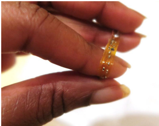
Fig. 7 Flexible conformal PDMS-packaged layer on capacitive proximity and touch sensing circuit
