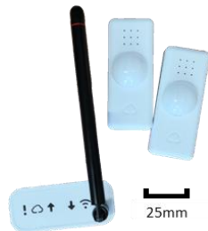
Fig. 3 The wireless PIR sensors [25] used in the study and the network interface controller (hub).
