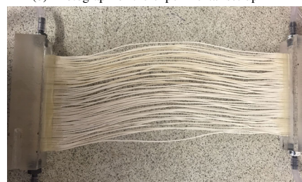
(c) Image of the membrane fixing and potting used to secure the hollow fibre membranes
