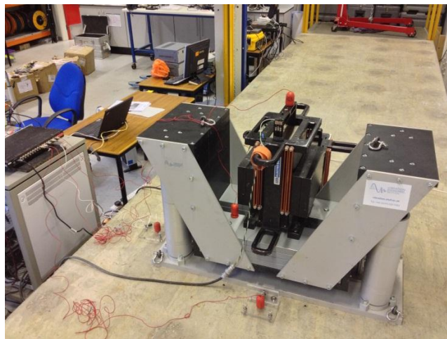
FIGURE 2.4: An application of electromagnetic proof mass actuators in civil structures: a hybrid tuned mass damper for floor vibration reduction. Reproduced from [36].
