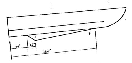
Skeg Area = 15.055 x a where a = 28.34  $\tan \theta$  and  $\theta$  = angle between L.E. skeg and hull.
