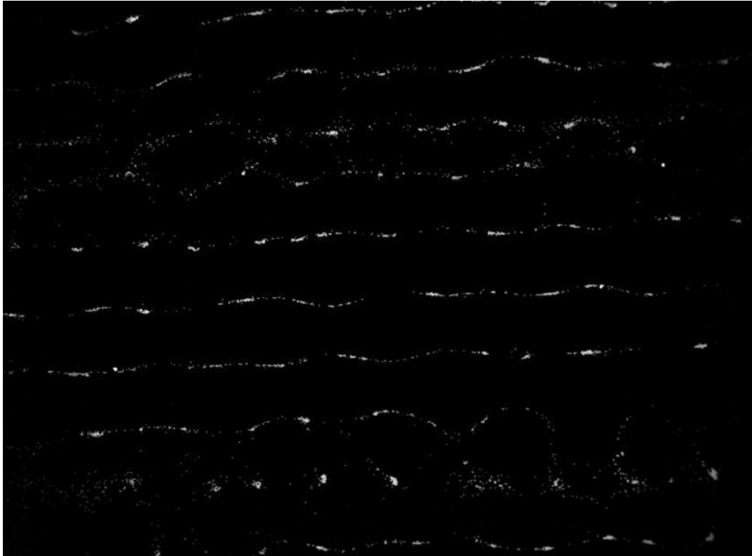
Figure 26- Example of particle final position in a planar resonator being driven at half-wave mode frequency. The half wave mode is disrupted by a non-controlled lateral cavity mode, dominating the final configuration of particles. (Particles are 10 \mu\text{m} polyester beads, cavity of 420 \mu\text{m} filled with water, driven at 1.72 MHz)
