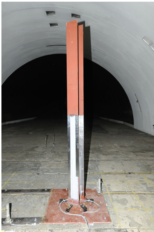
Figure 3. Cantilever I-section configuration in the ABT viewed upstream for the 30° I-section orientation.
