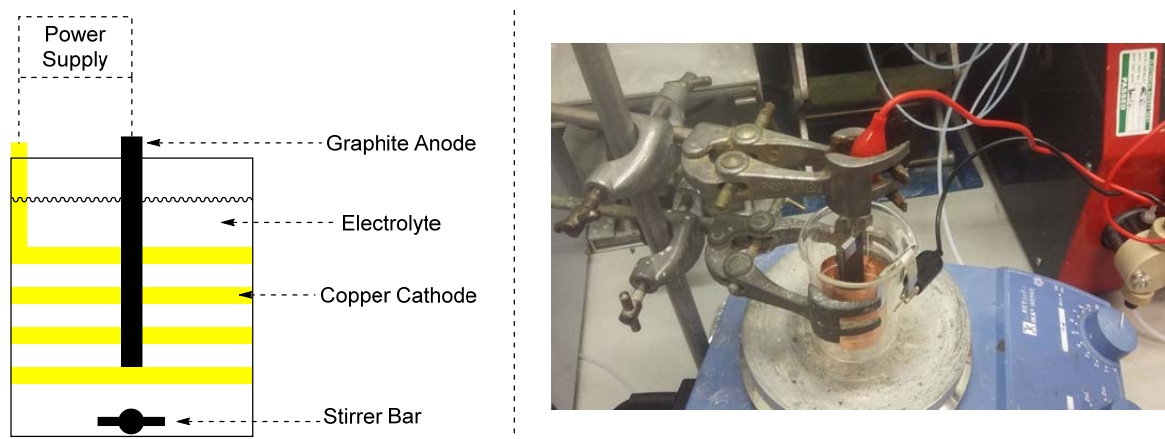
Figure 6.3: Left: Schematic representation of the beaker cell. Right: Picture of the setup in reality.
