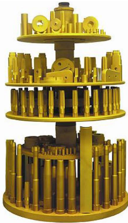
Figure 4: An example of TiN coated tool parts coated by CVD of \text{TiCl}_4 , \text{N}_2 and \text{H}_2 . 22
