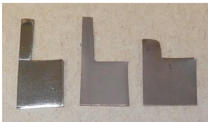
Figure 58: A photograph of vanadium based electrodes, showing vanadium metal (left), VN (middle), and thermally oxidised VN (left).
