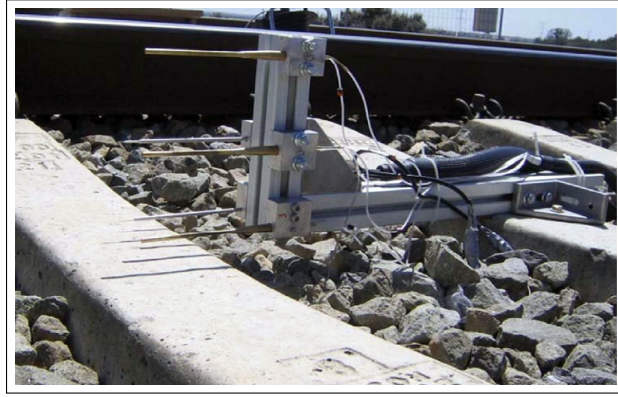
Figure 1.7: Pitot tubes and hot-wire anemometers installed on the track.
