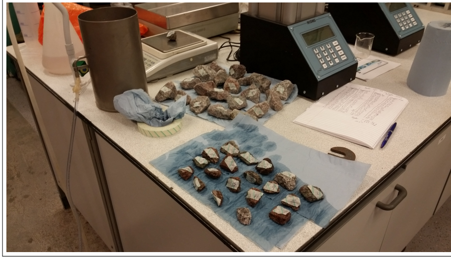
Figure 4.58: Eureka Can Experiment to measure volume of twenty large and twenty small granite particles.
