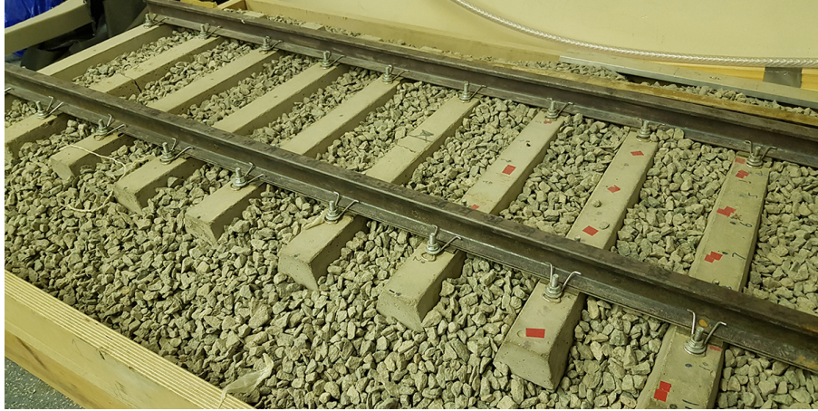
Figure 5.46: Scaled model (1:5) of ballasted track using mono-block sleepers. University of Southampton.
