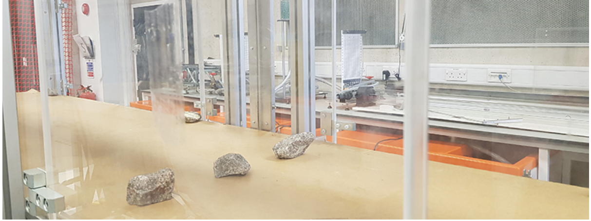
Figure 4.79: Wind tunnel setup to measure critical velocity to trigger ballast movement.
