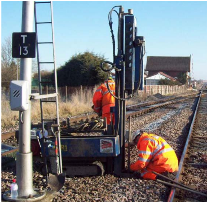
Figure 4.1: Windowless sampling rig in use AECOM Ltd. (2016)
