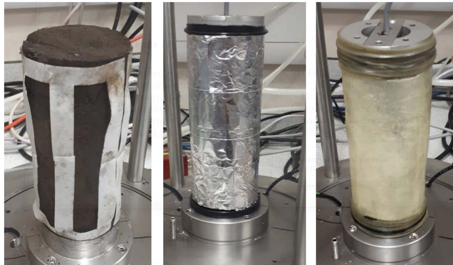
Figure 4.16: RC sample assembly - radial drain followed by latex membrane, greased foil strips and a second latex membrane.
