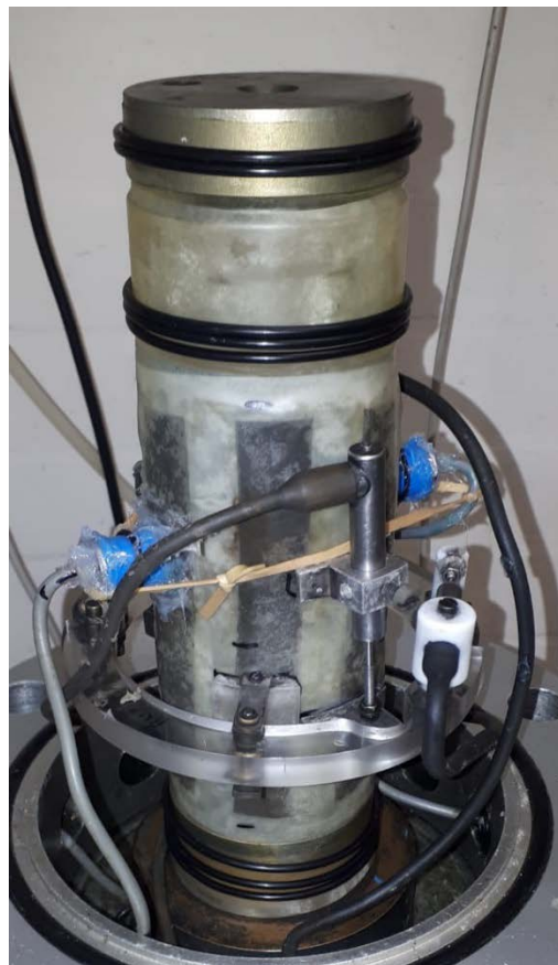
Figure 4.18: LVDT and bender elements (blue) set up on triaxial specimen.
