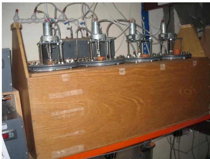
(b) Set of 5-L digesters in temperature controlled box
