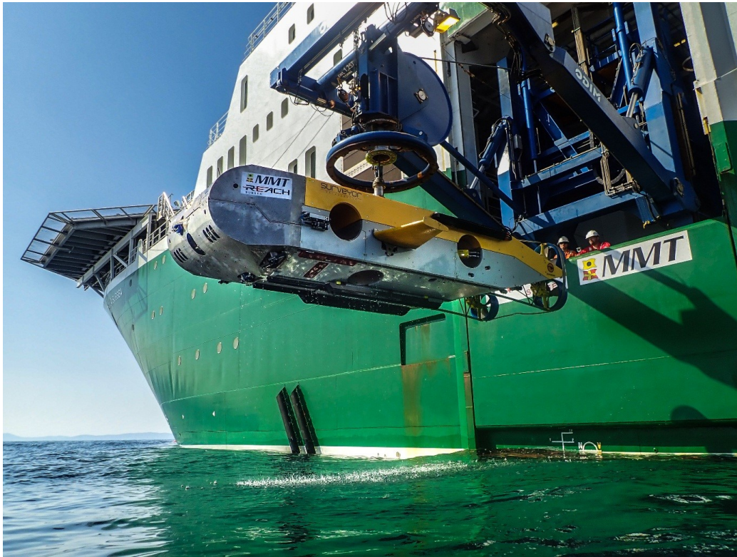
Figure 10: Image of SROV launched from MPSV Havila Subsea . Image the authors
