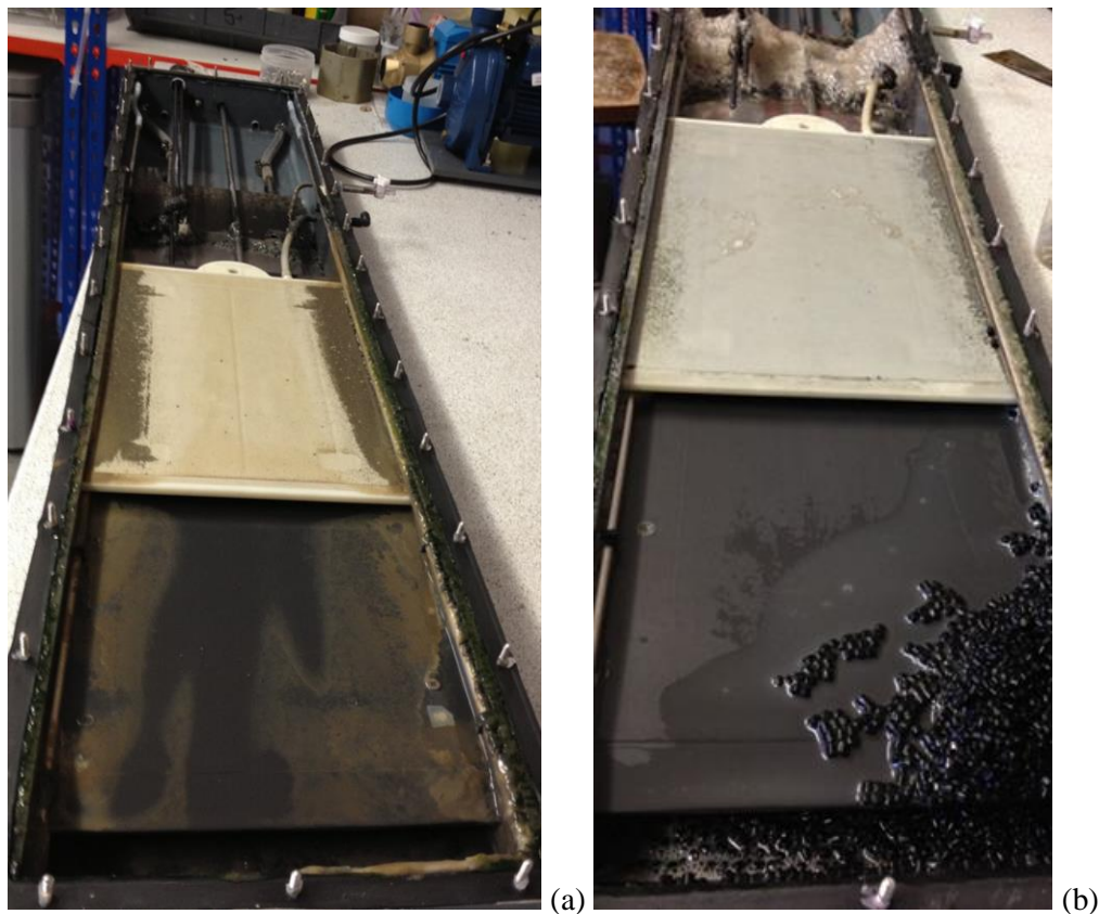
Figure 6-14 Fouling characteristics within the reactors after system termination (a) GSAnMBR and (b) MBAnMBR
