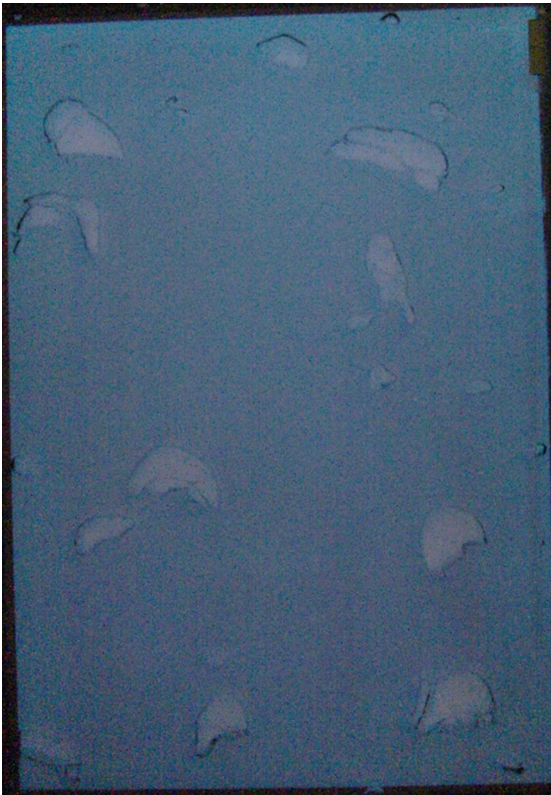
Figure 3-4 Original image of bubble flow in pseudo-2D thin channel (nozzle \varnothing 4 mm, 8 L min -1 sparging rate)
