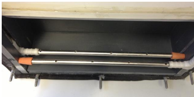
Figure 3-2 Nozzles and spargers arrangement for the case of equal nozzle sizes
