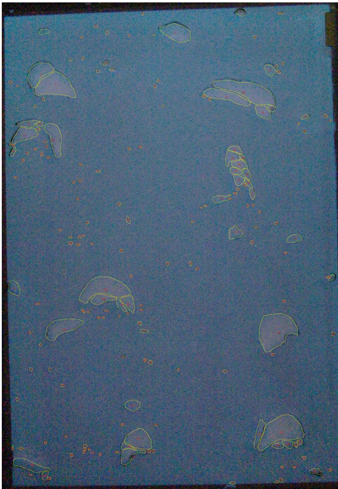
Figure 3-5 Analysed bubble perimeters (nozzle \varnothing 4 mm, 8 L min -1 sparging rate)
