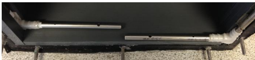
Figure 3-3 Nozzles and spargers arrangement for the case of Ø1.5 and 3 mm nozzle sizes
