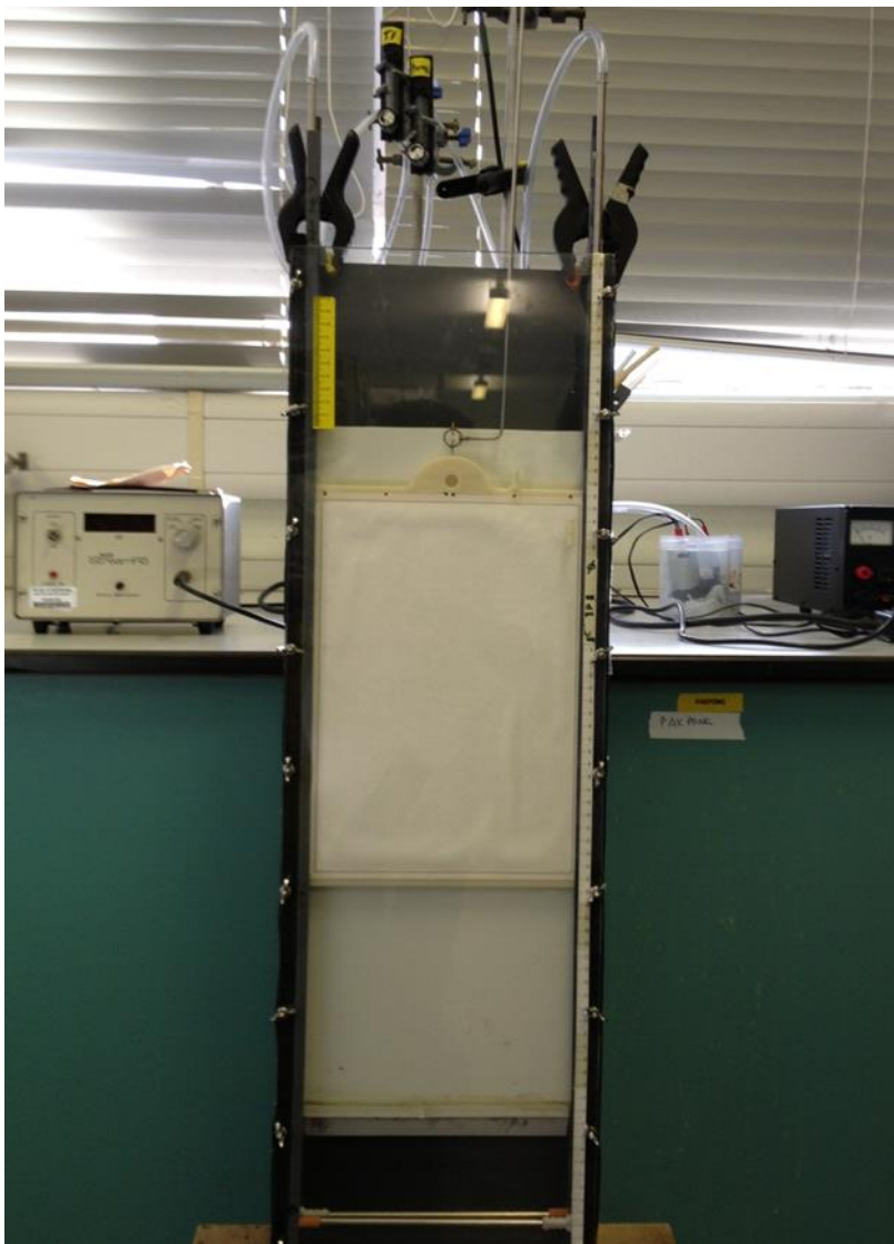
Figure 3-8 Flow velocity measurement apparatus set-up
