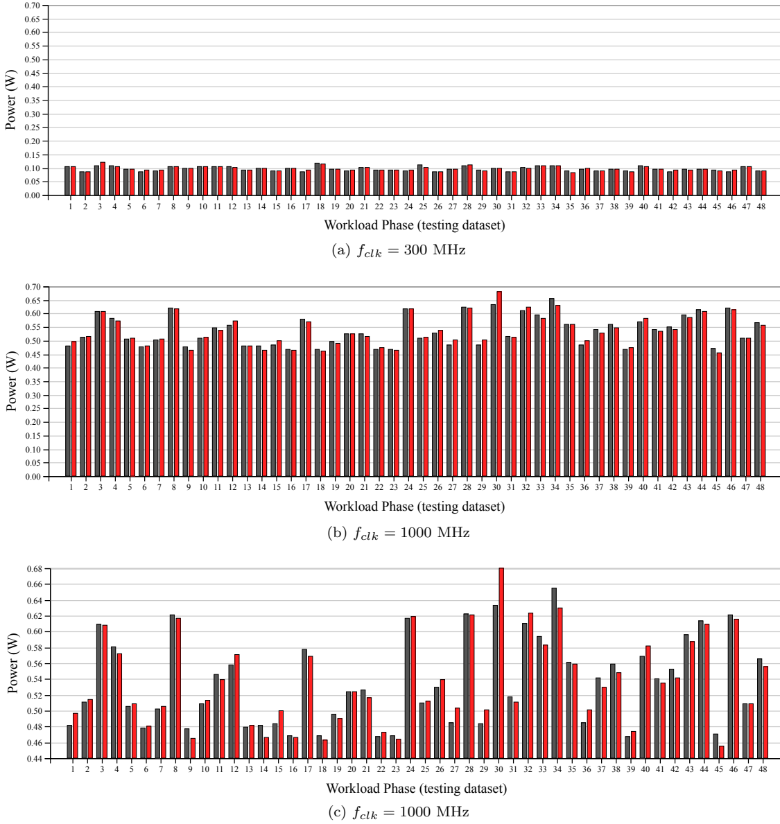
Figure 3.24: Cross-fold validation across all testing observations (Note that the observations are not consistent between plots of different DVFS levels as the workload phase selections are randomised).
