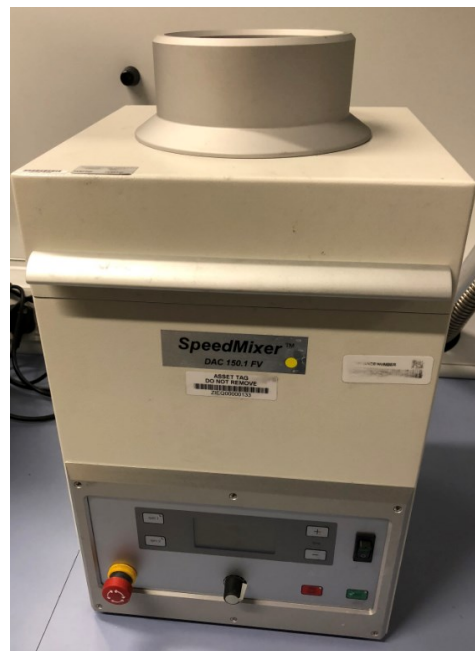
Figure 5-1: Speed mixer for mixing silicone and carbon black (DAC 150.1 FV-K, Hauschild Engineering).
