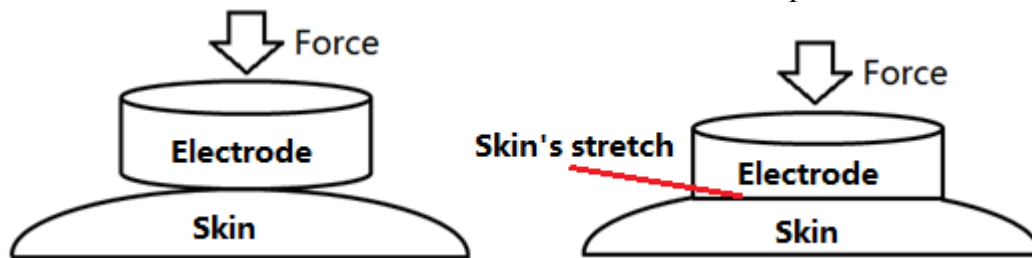
Figure 3-3: Force applied to the electrode (before application and immediately after).
