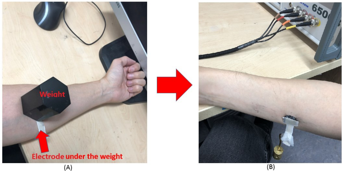
Figure 5-18: Adhesion test for MED-6350 electrode. (A) Before testing, applying force to provide a full contact. and (B) Testing the adhesive force in the vertical direction.
