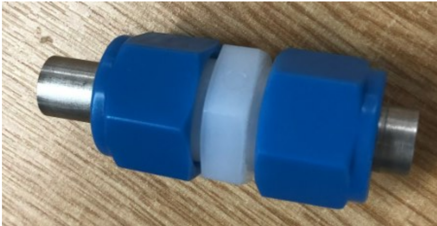
Figure 5-6: Fitting tube for measuring the permittivity of MED-6350.
