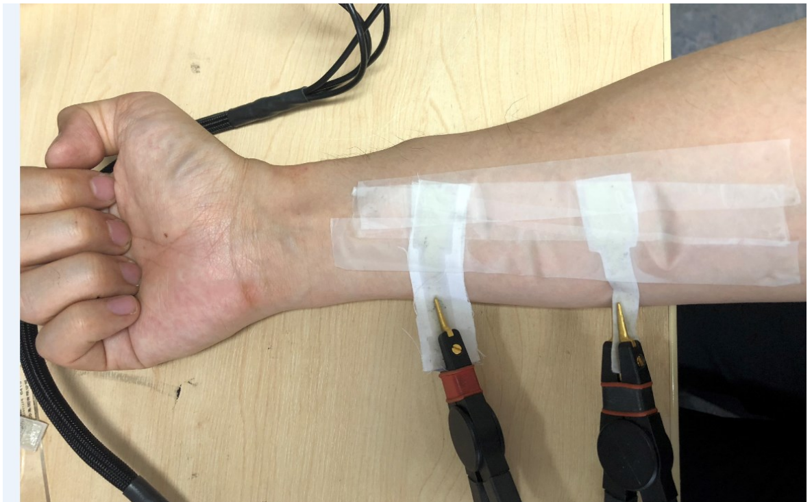
Figure 4-12: skin-electrode impedance measurement setting for silver electrode pair (two electrodes are connected impedance analyser).
