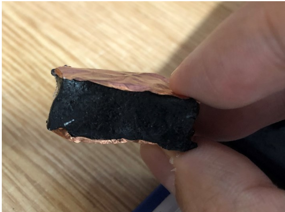
Figure 5-3: MED-6350 placed into copper plates, size of copper plates: 3 cm × 3 cm and size of MED-6350: 3 cm × 3 cm × 1 cm.
